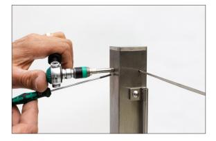
Turn the rope tensioner with a ratchet wrench and fix the rope tensioner with M3 screw at one of the four thread positions. Then cut the rope ends on the other fence side to the appropriate length (approx. 15cm longer than the end of the post). After that insert the rope into the tensioner and bring it to the desired or required final tension. Fix it again with M3 screw.
